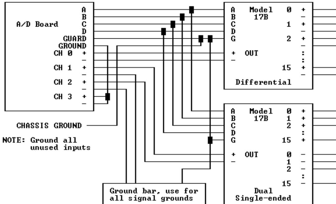
Read differential inputs 0-15 at A/D channel 0
