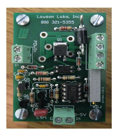
Output up to 2 amps at 8 to 24 volts, isolated or not
